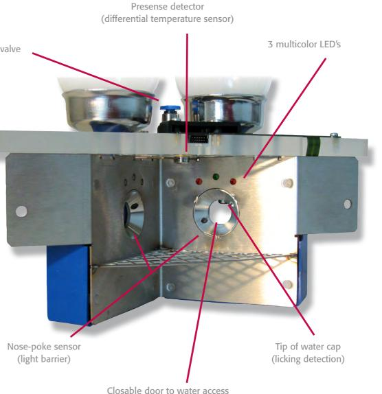
• RFID antenna - identifies the animal (transponder) entering a corner • Temperature-sensitive presence sensor - detects start, duration and end of corner visits • IR light beam at the door to water water access - detects nose poke instances · Lickometer - detects the number and duration of tongue-contacts with drinking nozzel
