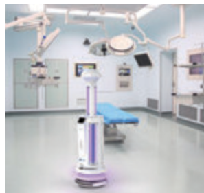
Multi-mode combined disinfection - ultraviolet catalyzed hydrogen peroxide decomposition
